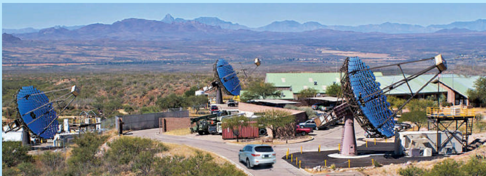
Photograph 8.1 Cherenkov telescope on Mount Hopkins, United States of America used to detect cosmic rays
