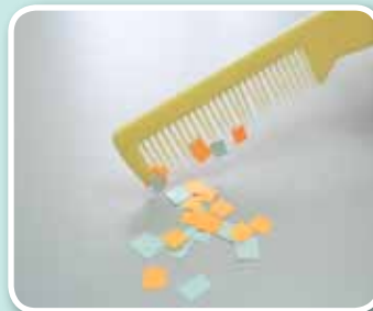
(c) Tiny pieces of paper are attracted to a charged plastic comb
