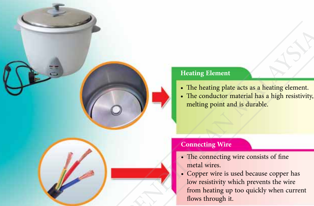
Figure 3.22 Applications of resistivity in an electric rice cooker
