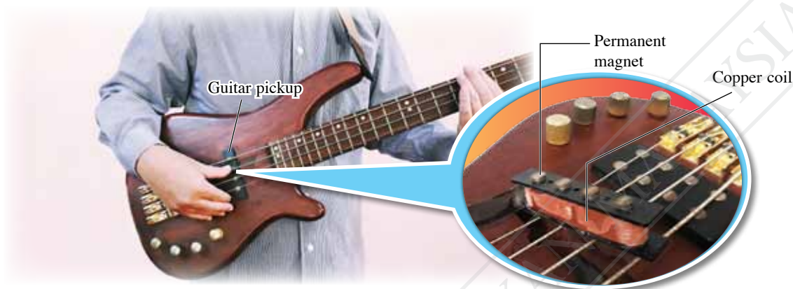
Photograph 4.4 Components in an electric bass guitar pickup
