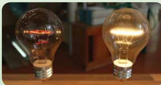
(c) Thermal radiation in light bulbs at different temperatures
