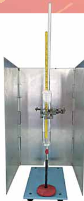
Photograph 2.2 Apparatus set-up for measuring calorific value of food
