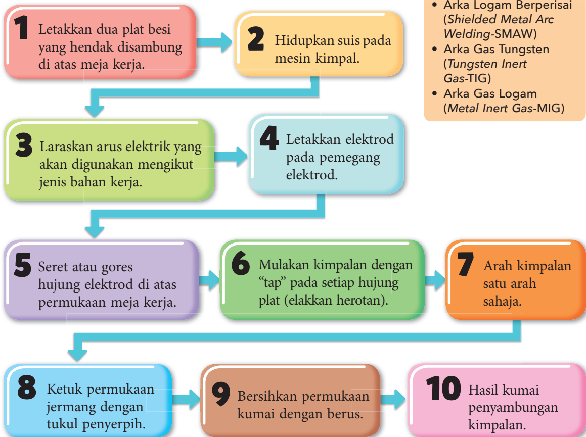
Rajah 5.3.13 Proses kerja kimpalan arka logam berperisai (SMAW)
