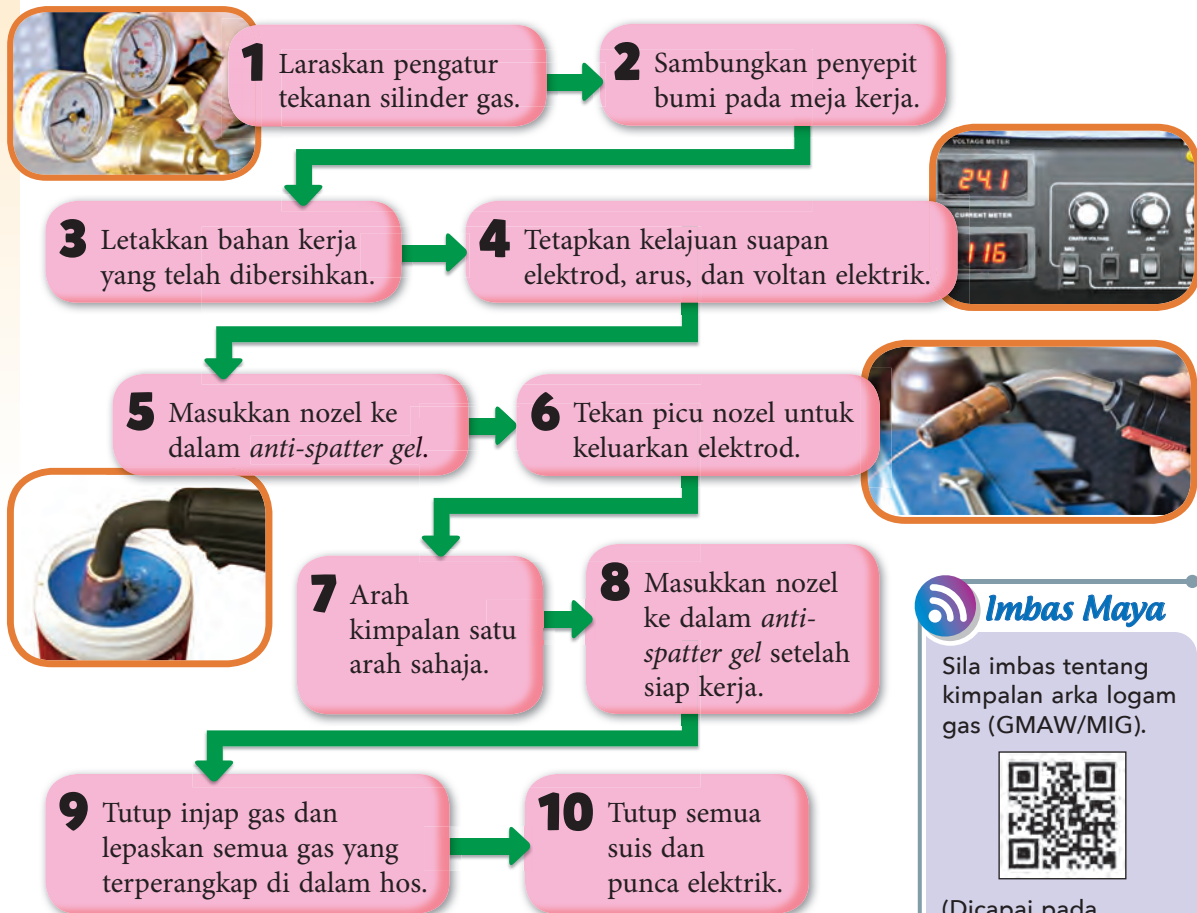
Rajah 5.3.15 Proses kerja kimpalan arka logam gas (GMAW/MIG)
