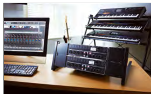
Foto 1.13 Contoh rackmounted audio interface
