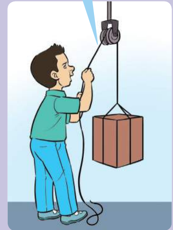
pulley to lift a load
